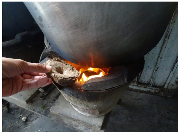
Photo 10. Tests: Feeding big pellet to mud cook stove
