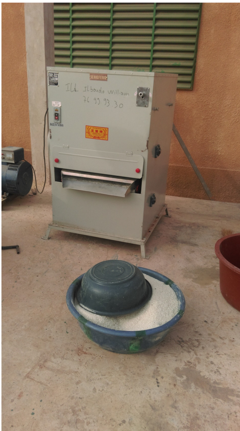
Figure 23 Rice cleaning machine (removal of stone)
