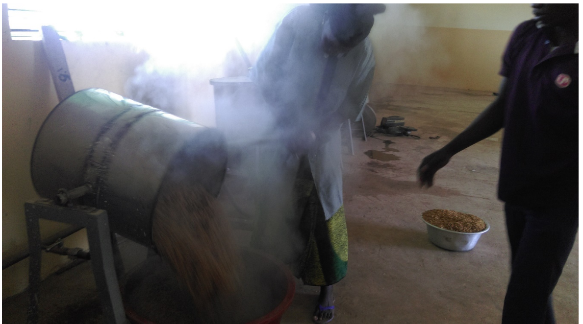
Figure 20 Rice steaming (10 minute per 75 kilo)
