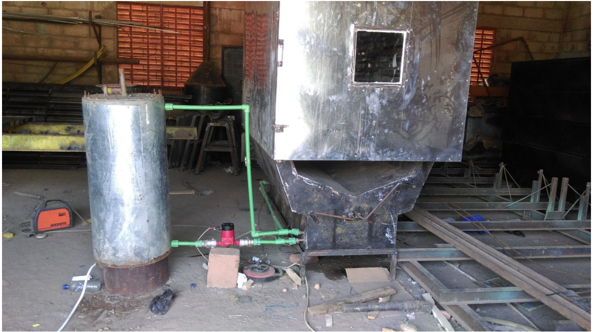
Figure 19 Test of mango dryer with indirect heat
