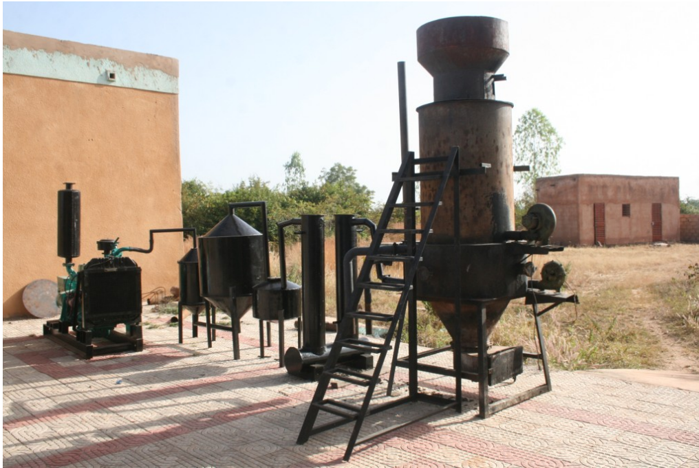
Figure 5 Installation of genset and gasifier for electricity
