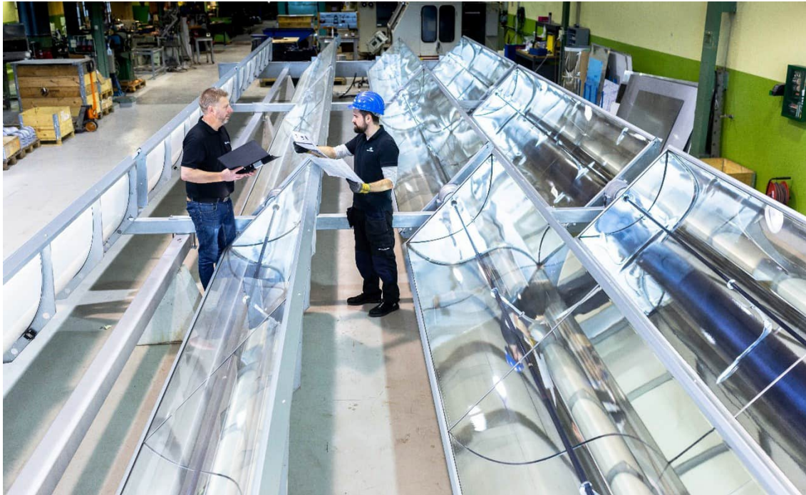
Christer Pekkala and Krzysztof Adamczyk undertaking testing of tracking system in Sweden before shipping of solar collectors in Milestone 1 to Kenya Photo: Absolicon
