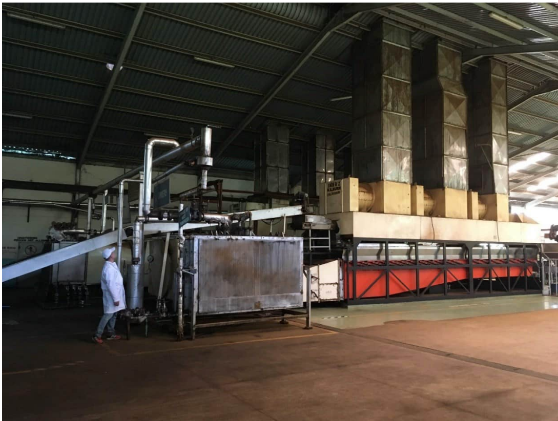
Stefan Jonsson, Glofin, inspecting the air intake where the preheater for the tea dryer at Chelal Tea factory will be installed. Photo: Absolicon
