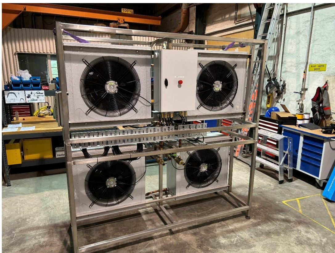
Fan unit to be installed at the tea dryer in Chelal tea factory waiting for shipping. Photo: Absolicon
