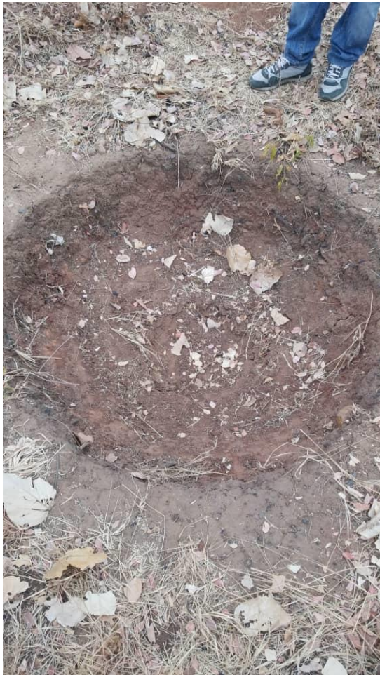
Biochar production flame curtain kiln after finishing the biochar making and covering with wet sand. Photo by Gibson Simosokwe
