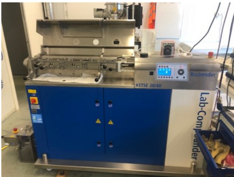
Ketse 20/40, twin-screw extruder from Brabender GmbH at the feed technology laboratory at the Swedish University of Agricultural Sciences (SLU), Uppsala, photo Aleksandar Vidakovic
